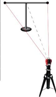
The **ASME B89.4.19-2006 standard** prescribes a series of tests for evaluating the performance of spherical measurement systems. These values represent the Maximum Permissible Error (MPE) between a verified Scale Bar and the expected performance of the instrument.
