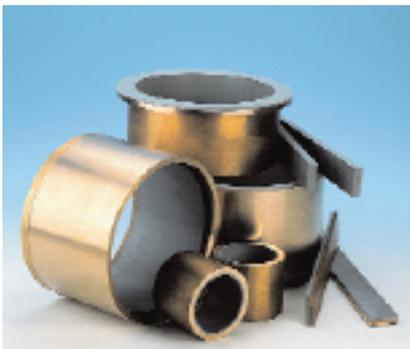
**Thordon HPSXL (grey) is designed for higher pressure applications as the bearing component in HPSXL TRAXL bearings (HPSXL bonded in a metallic shell).**
