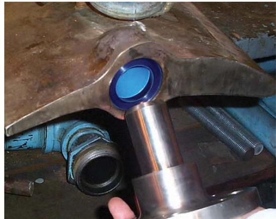
Both HPSXL and ThorPlas® are easily machined and can be supplied either finished to final sizes provided by the customer, or with overbuild to facilitate line boring after installation to correct the misalignment and dimensional inconsistencies often encountered during turbine rehabilitation.
