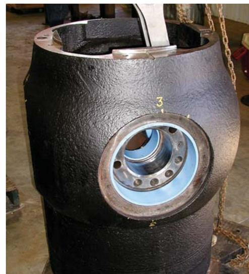
**Alabama Electric installed ThorPlas® runner blade trunnion bushings for their Kaplan turbine**
