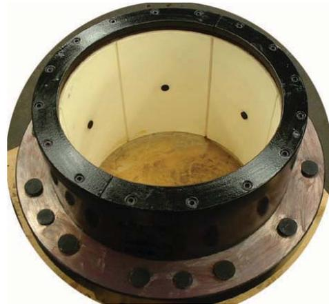
Thordon can be specified as an upgrade for rubber or other non-metallic bearings in existing water-lubricated bearing systems or as a complete conversion from sealed oil or grease lubricated systems to pollution-free water lubrication. Although elastomeric in nature, Thordon bearings, particularly SXL are stiffer than rubber and capable of supporting higher loading. A high degree of resilience, however, is still maintained and running clearances similar to rubber are possible.
